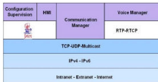
Figure 2. AudioLAN architecture within the Simulation Environment
